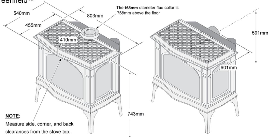
The 168mm diameter flue collar is 768mm above the floor
