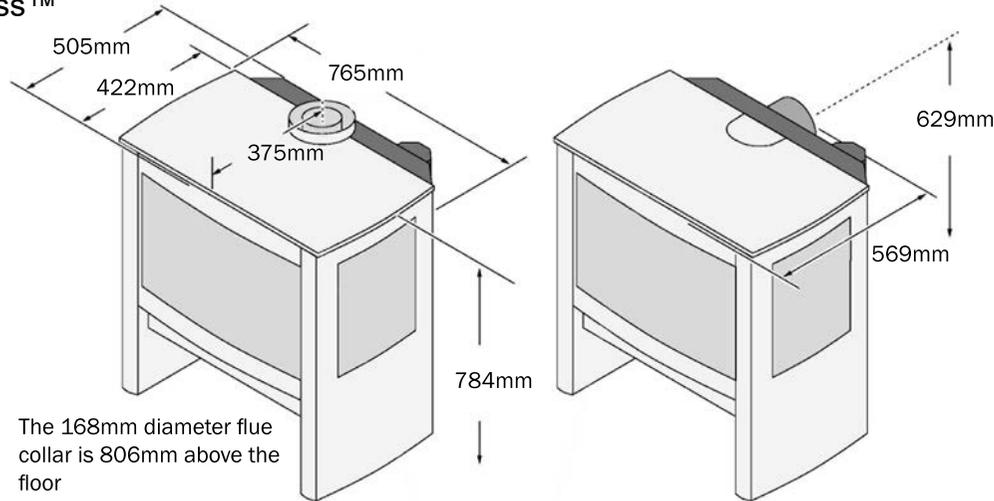
The 168mm diameter flue collar is 806mm above the floor
