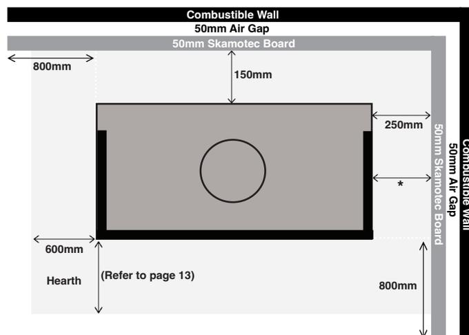
The Skamol boards should extend to a minimum height of 1800mm from the hearth when using a triple skin flue kit OR all the way to the ceiling when using a single skin flue kit (refer to page 17). When using Skamoltec board with a 50mm air gap behind, it must also be ventilated for natural air flow circulation, (refer to page 15 & 16 for ventilation requirements).
