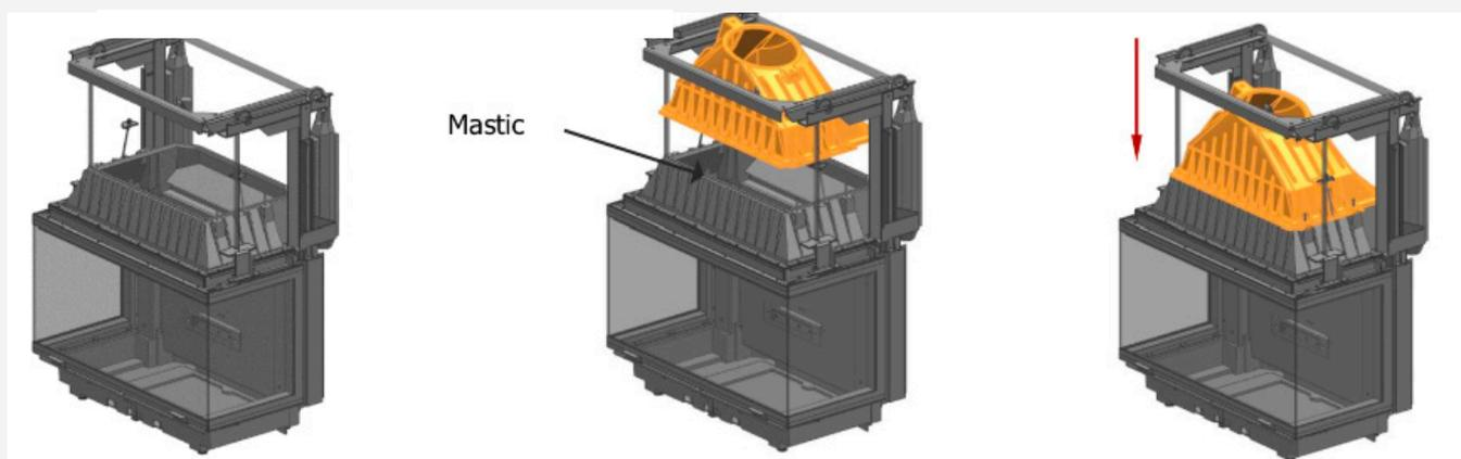
1. Position the gather onto the firebox, then carefully apply refractory sealant (mastic) to all supports and interlocking joints of this assembly
