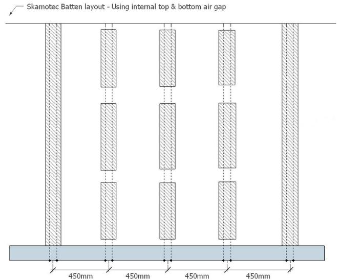
The 25mm top and bottom air gap must extend the full width of the Skamotec cavity and can be left open to create a shadow line effect, or alternatively can be faced with a metal grill/vent
