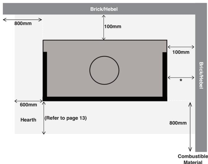
A minimum 110mm solid brick/hebel thick wall should extend a minimum height of 1800mm from the hearth when using a triple skin flue kit or to the ceiling when using a single skin flue kit.
