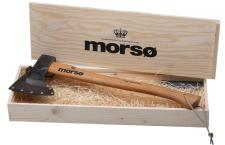
With a beautiful linseed-oiled handle made from USA Hickory wood which is hard and dense with exceptional flexing strength, and a traditionally forged high grade carbon steel blade, the Morsø Axe comes with a genuine leather sheath and sharpening stone. The Morsø Axe head is forged from C45 high grade carbon steel with a Rockwell hardness of approximately 53-56HRC (According to DIN 7287/B).
